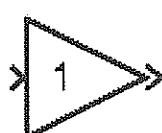
The Gain block multiplies the input by a constant value (gain). The input and the gain can each be a scalar, vector, or matrix. Specify the
