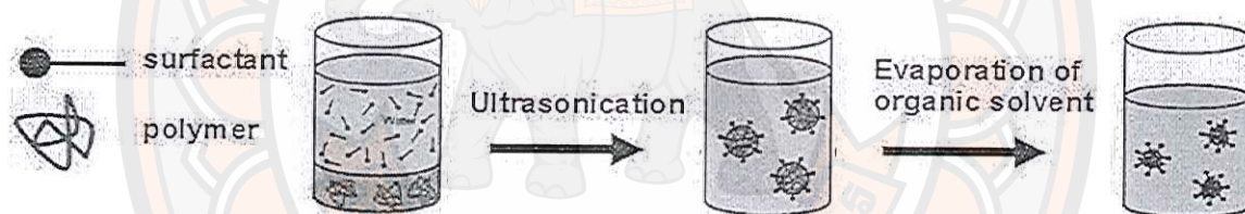
Figure 30 Process of miniemulsion polymerization [28]
