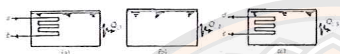
Fig 1. The three stage in a simple heat storage, charging period (a), Storage period (b), and discharging period (c) [8].
