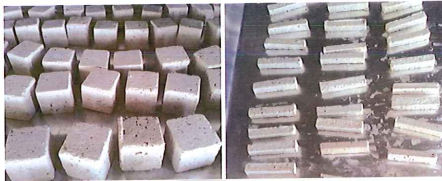
Figure 15 Configuration of tested samples of concrete
