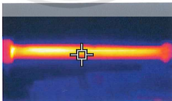
Figure 53 Temperature distribution in the cylinder pipe at 100°C
