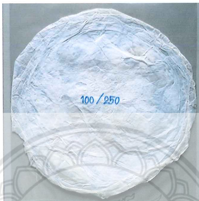
Figure 31 Freeze-dried BC at the volume of 100/250 (v/v) using stainless container
