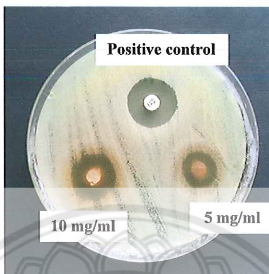
Figure 89 The diameter of clear zone of BCP at the concentration of 5 and 10 mg/ml and positive control against S. aureus
