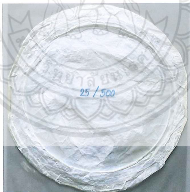
Figure 32 Freeze-dried BC at the volume of 25/500 (v/v) using stainless container
