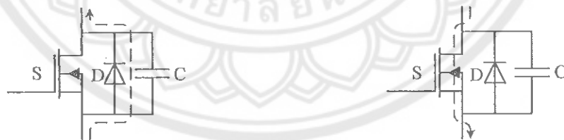
(a) Switch OFF ready for ZVS ON
