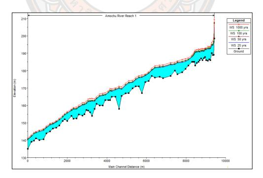
Figure 11 Water surface profile of different return period flood
