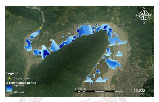
Figure 16 2-year flood extend for Amochu River in Phuntsholing City
