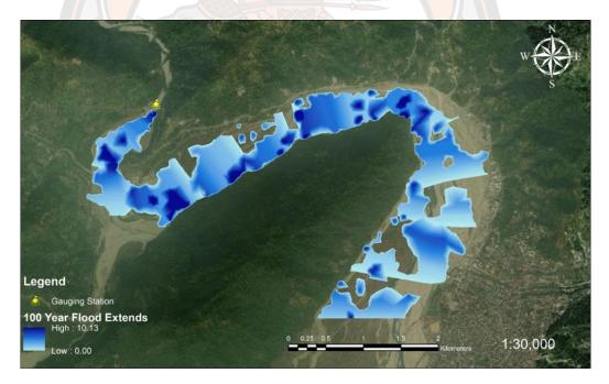
Figure 21 100-year flood extend for Amochu River in Phuntsholing City
