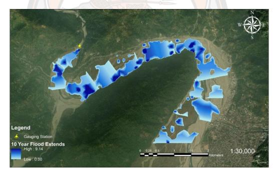
Figure 25 10-year flood extend for Amochu River in Phuntsholing City
