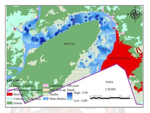
Figure 31 100-year flood effect on the of study area using LULC 2016
