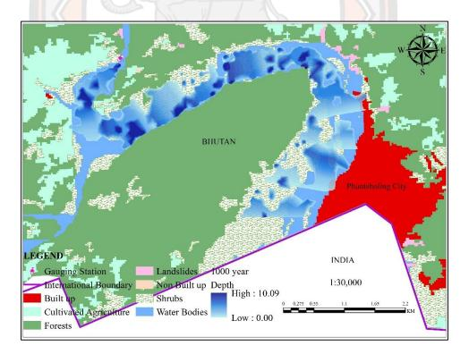
Figure 32 1000-year flood effect on the of study area using LULC 2016
