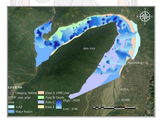
Figure 41 1000-year flood effect on the study area using future city master plan
