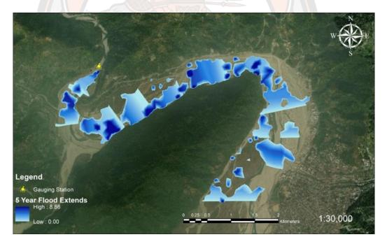
Figure 17 5-year flood extend for Amochu River in Phunstholing City
