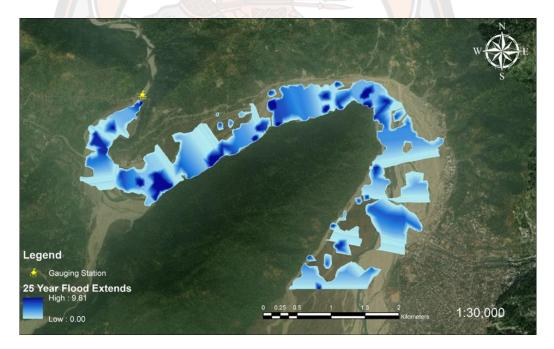
Figure 19 25-year flood extend for Amochu River in Phuntsholing City
