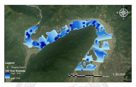
Figure 28 100-year flood extend for Amochu River in Phuntsholing City
