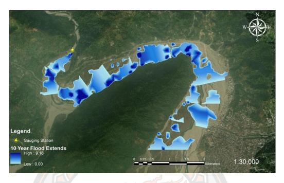
Figure 18 10-year flood extend for Amochu River in Phuntsholing City
