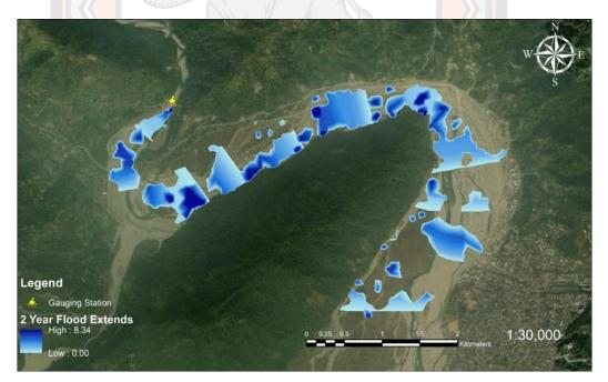
Figure 23 2-year flood extend for Amochu River in Phuntsholing City
