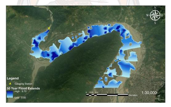
Figure 27 50-year flood extend for Amochu River in Phuntsholing City
