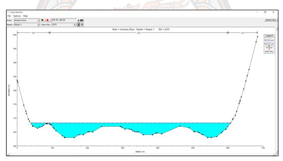
Figure 13 Graphical representation of cross section for steady flow
