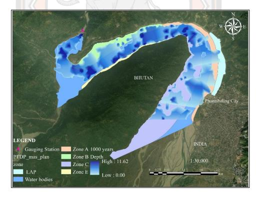
Figure 46 1000-year flood effect on the study area using future city master plan
