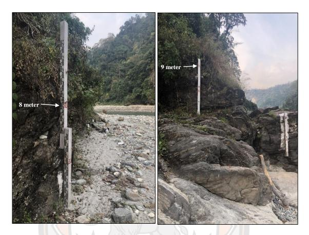
Figure 15 Actual depth value of 2009 extreme flood event at 8m to 9m observed at Doyagang gauging station
