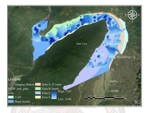
Figure 43 25-year flood effect on the study area using future city master plan
