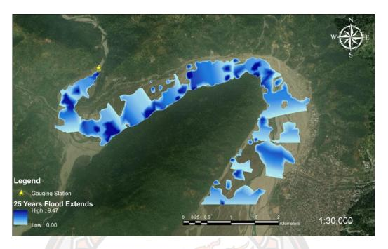
Figure 26 25-year flood extend for Amochu River in Phuntsholing City
