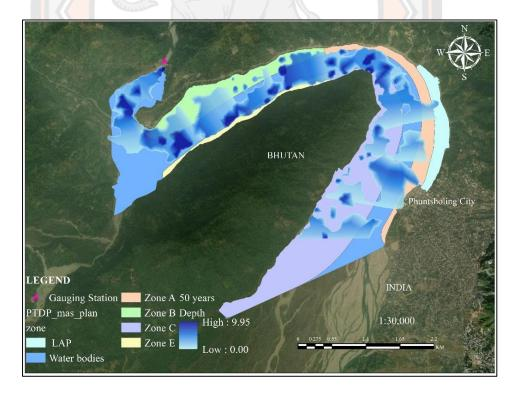
Figure 44 50-year flood effect on the study area using future city master plan
