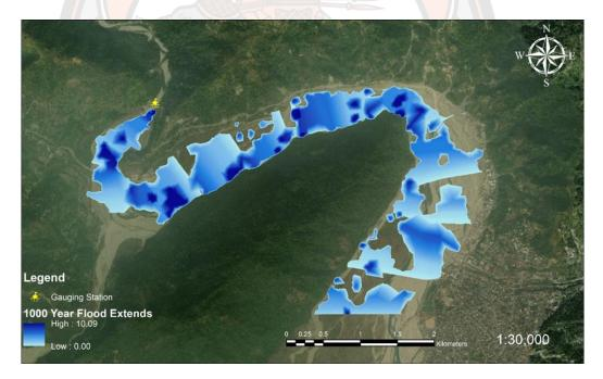
Figure 29 1000-year flood extend for Amochu River in Phuntsholing City
