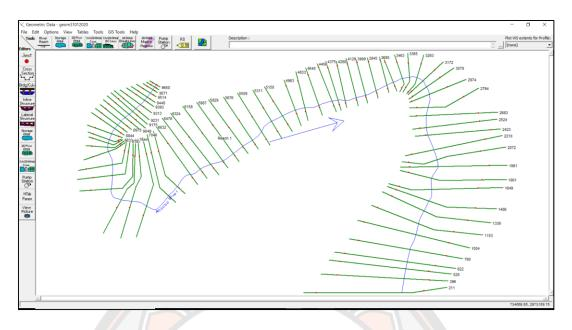
Figure 12 River geometry for the steady flow analysis
