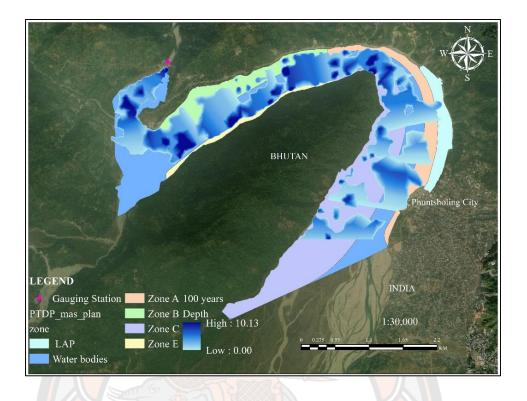
Figure 45 100-year flood effect on the study area using future city master plan
