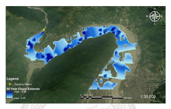
Figure 20 50-year flood extend for Amochu River in Phuntsholing City
