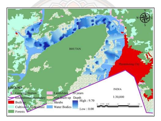
Figure 30 50-year flood effect on the of study area using LULC 2016
