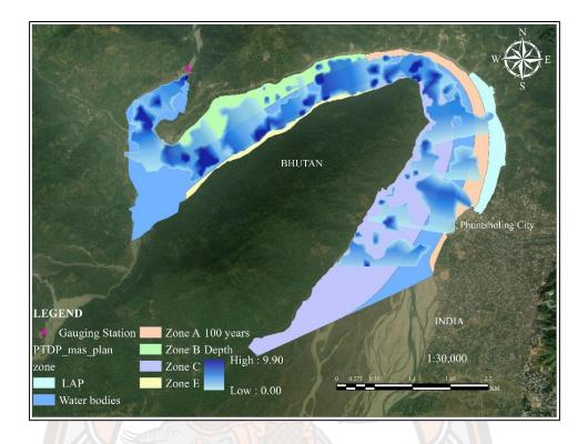
Figure 40 100-year flood effect on the study area using future city master plan
