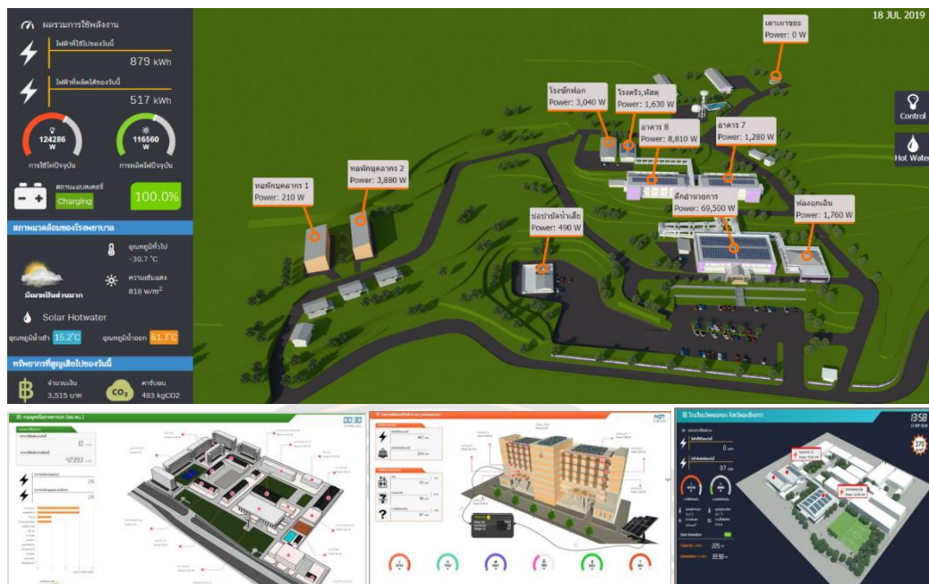
Figure 39 The implementation of an example of the aBEMS-IoT in the actual building
