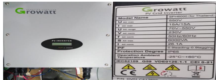
Figure 29 The 5 KW Growatt PV Grid Inverter (Thailand)
